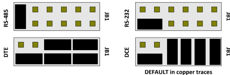
The board is configured as RS-232 DCE to allow use of a 1 to 1 cable between the CFSound and a PC. This configuration is established by copper jumpers on the bottom of the board between the JB1 pins.
